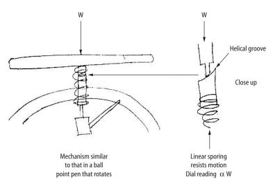
Above: A sketch taken from a student's sketch pad showing a design based on a biro (ballpoint pen) deploy-retract mechanism.
